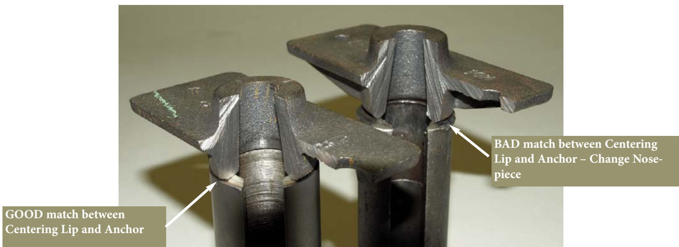
Fig. 4 - Ensure that the centering lip on the nose piece of the jack is not excessively worn.
